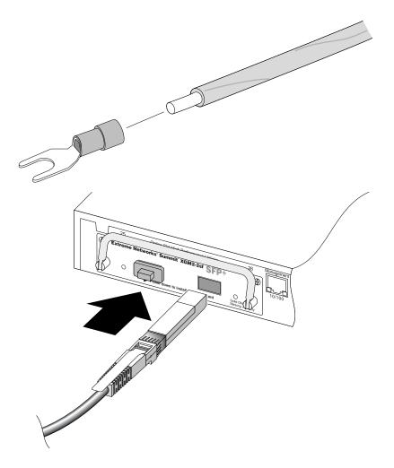
Figure 9: Connecting an SFP+ Direct-Attach Cable to an XGM2-2sf Option Card (Cable A and Cable B)
